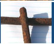
**Pitted Rust** Not suitable for use as concrete reinforcing
