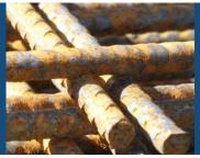
**Slightly Rusty** Suitable for use as concrete reinforcing
